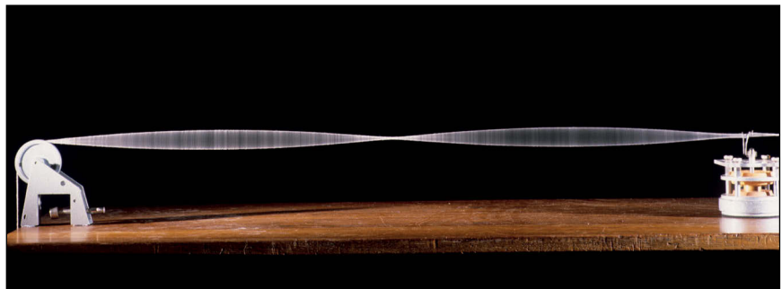
Figure 4.64 A string vibrating.
