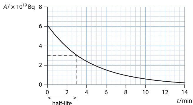
Figure 7.9 The activity of thallium decreases exponentially with time. You can also use this graph to determine half-life.
