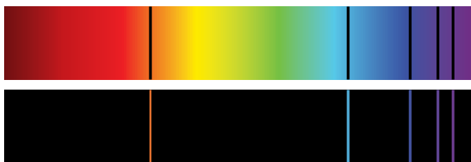
Figure 7.5 The absorption spectrum of hydrogen (top) and the emission spectrum (bottom). The emission lines and the absorption lines are at the same wavelength.
